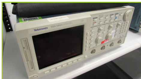
TEKTRONIX TDS554A COLOR FOUR CHANNEL DIGITAL PHOSPHOR OSCILLOSCOPE. OUTPUT-500 MHZ, 1GS/S, INPUT- 90-250V, 47-63 HZ
