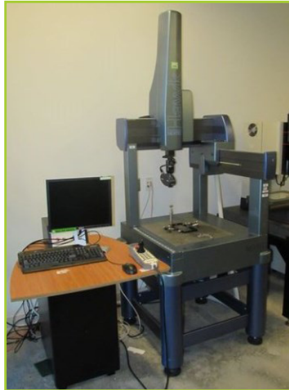
COORDINATE MEASURING MACHINE. NEXTEC HAWK, WITH RENISHAW M1H PROBE, NEXTEC WIZPROBE, PENDANT, & COMPUTER, YEAR 2001
