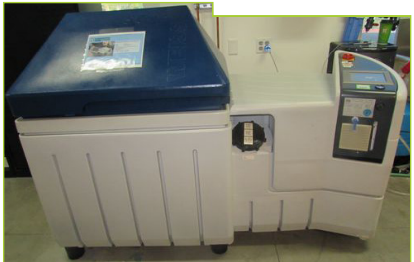
WEISS TECHNIK SC 450 ALTERNATING CLIMATE TEST CHAMBER. 34" X 23-1/2" X 28-1/2" CHAMBER
