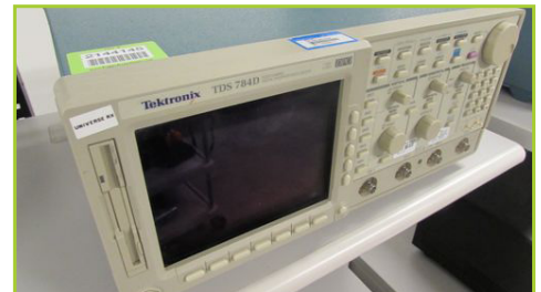
TEKTRONIX TDS784D FOUR CHANNEL DIGITAL PHOSPHOR OSCILLOSCOPE. OPTION 2M
