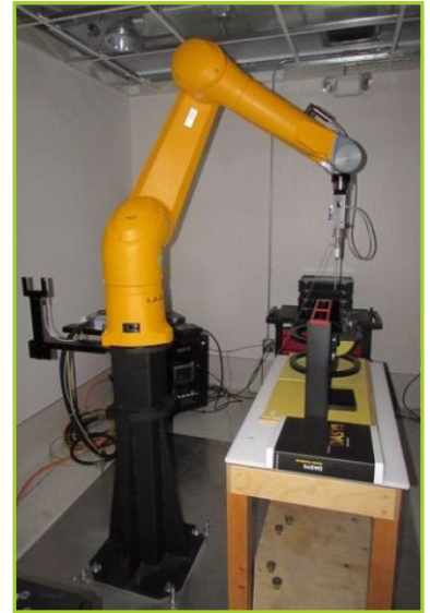
SPEAG (STAUBLI) TX90 XLSPEAG 6-AXIS ROBOT. DASY5, WITH SPEAG AMMI MEASUREMENT SERVER, CS8C CONTROLLER, PENDANT, COMPUTER, & ASSORTED PROBES, YEAR 2012
