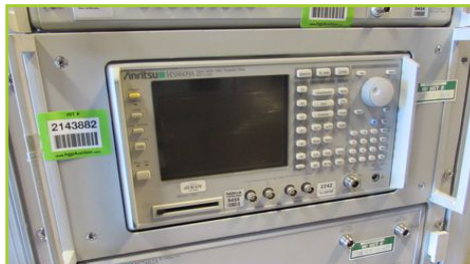
ANRITSU MS8609A DIGITAL MOBILE RADIO TRANSMITTER TESTER OPTIONS 01, 08, 04, & 47, OUTPUT- 9 KHZ-13.2 GHZ
