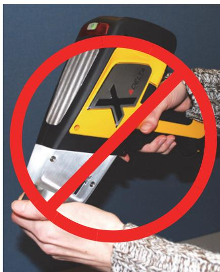
**Figure 2-7 Bad testing technique – Without dosimeter**
