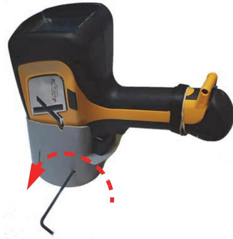
Figure E-7 Loosening the set screw
