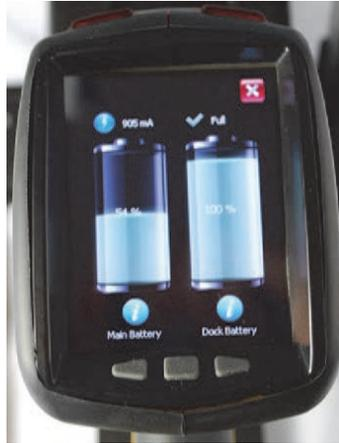
**Figure 3-2 Battery charge status**
