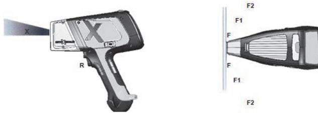
**Figure 10-1 DELTA radiation profile – Handheld instruments**
