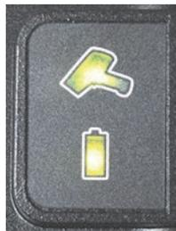
**Figure 3-6 Both batteries fully charged**
