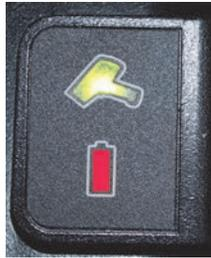
**Figure 3-5 Battery indicator turned on (red)**
