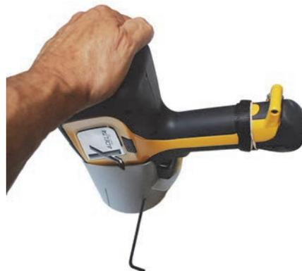
**Figure E-5 Analyzer properly seated and fastened**
