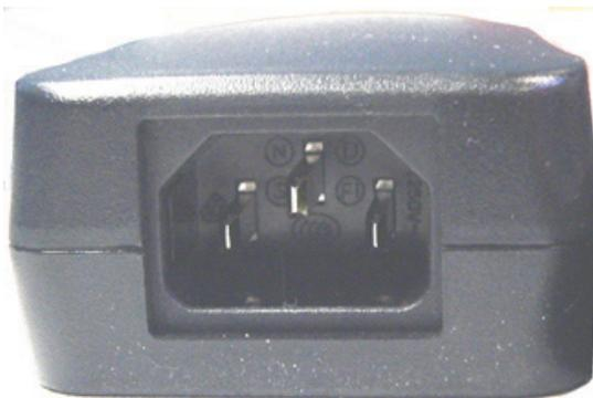
**Figure 3-15 Switching AC adaptor's male receptacle**
