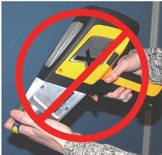
**Figure 2-6 Unsafe testing technique**
