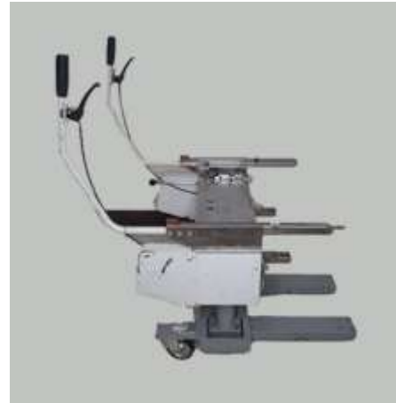
M6 Pallet Change Unit (Bucket Type)
