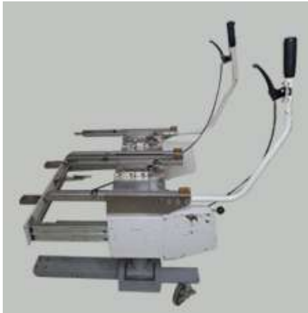
M3 Pallet Change Unit (Bucket Type)
