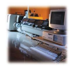
**Line Control Box** - Provides real-time changeover assistance, performance monitoring, feeder management assistance, and on-board error recovery features to maximize utilization on the factory floor.
