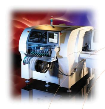
Equipped with two 7-spindle FlexJet3 placement heads and two upward looking cameras for large component image capture, this platform provides high-speed IC placement for high-volume lines or serve the role as a line balancer by off-loading chip placement in lower volume environments.
