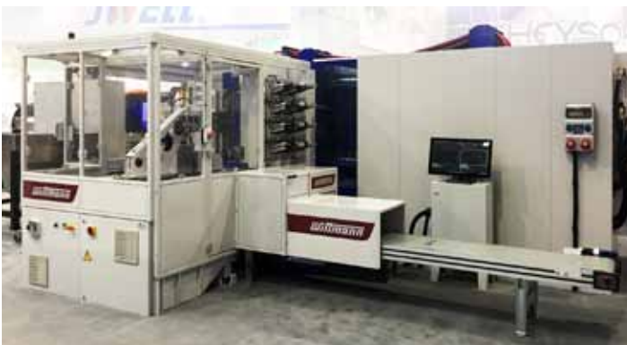
W837 Complete cell including camera control and stapling unit for food containers.
