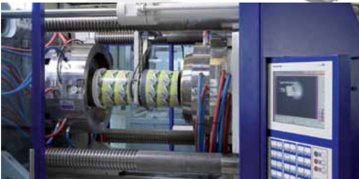
Example of a vertical production cell in the field of packaging: manufacturing of paint buckets.
